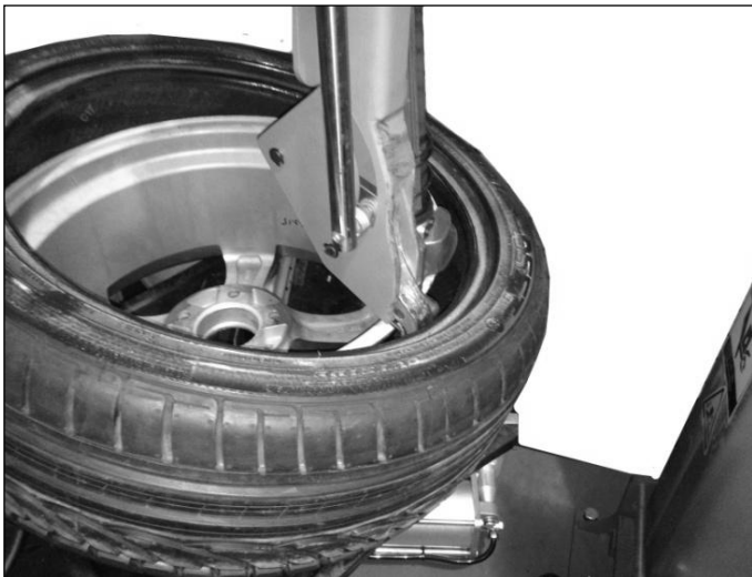
5.2.9 Use your hand to rise up the outside of the tire and press upward tool hook handle to hook up the tire.
