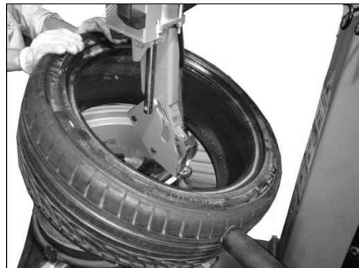
5.3.2 Clockwise rotate the turntable to drive the rim.
