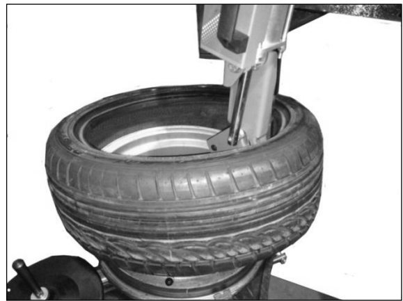
5.2.10 Step down the main shaft rotate switch to make the turntable drive the tire clockwise rotate.
