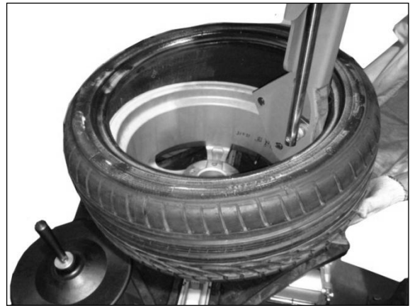
5.2.10 Step down the main shaft rotate switch to make the turntable drive the tire clockwise rotate.
