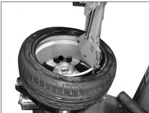
5.3.3 As the figure shown, press the tire press roller and the tire presser under the edge of the rim.
