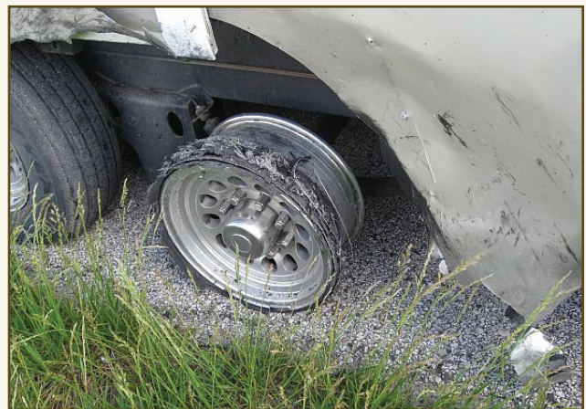
A tire blowout can destroy the wheel, damage the trailer, or cause the driver to lose control.
