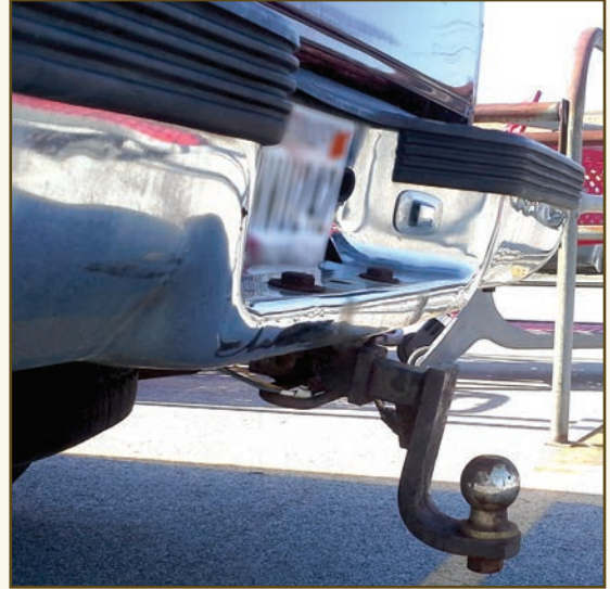
This hitch was damaged by too much tongue weight.
