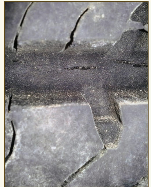
Cracks do not always appear in the tire wall. These cracks formed in the tread groove of a 10-year old tire with plenty of tread left. As the integrity of the tire decreases, the odds of a failure increase.
