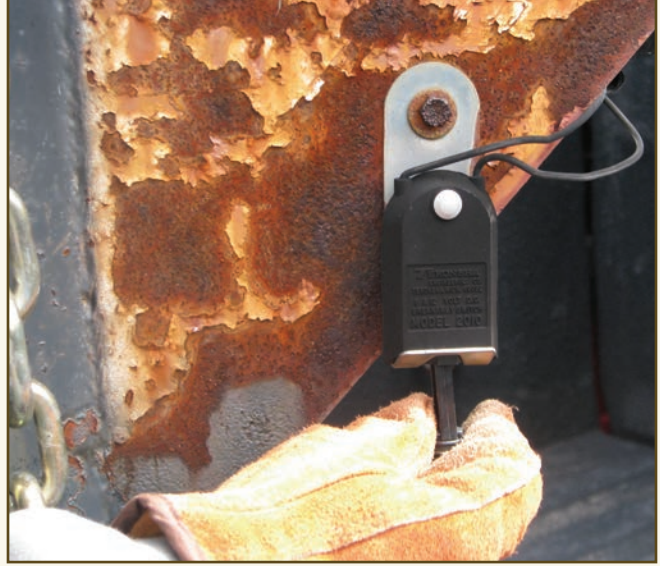
Pulling out the insert or pin of an emergency system will set the trailer brakes.
