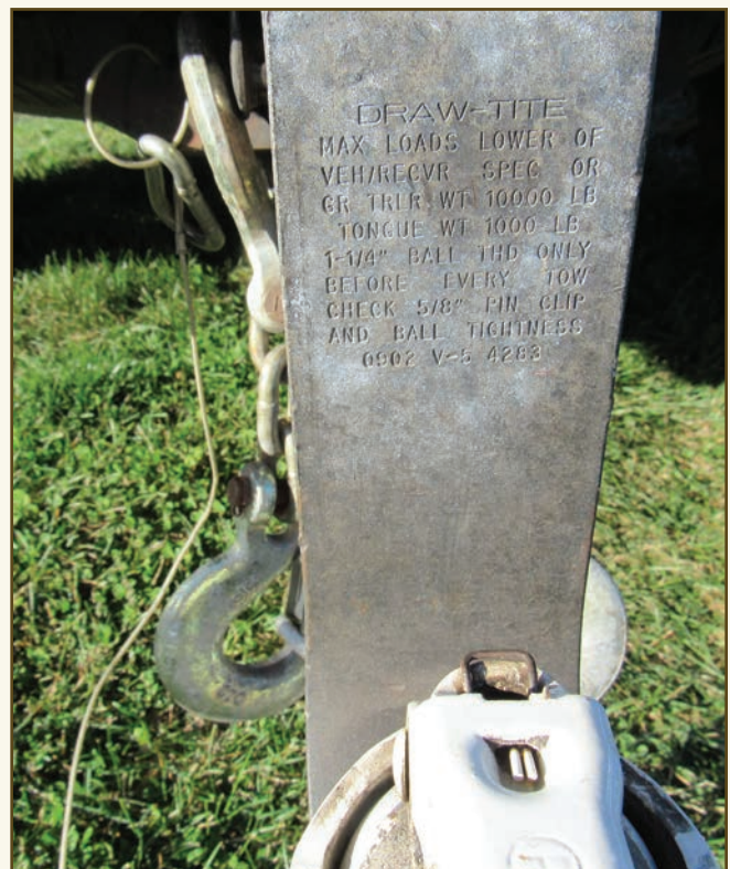
This insert is rated for pulling 10,000 pounds and a tongue weight of 1,000 pounds.
