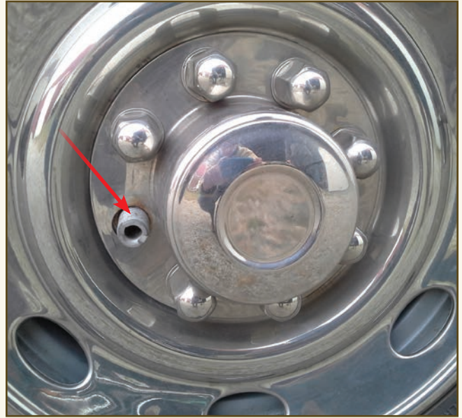
This photograph shows a hubcap with the locking nut removed. Now the hubcap can be removed to access the lug nuts and wheel studs to change a flat tire.
