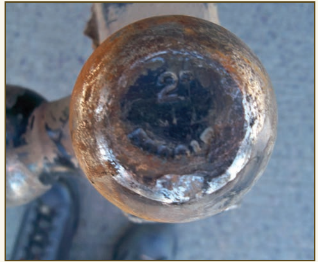
Lawsuits and settlements are often won or lost based on the condition of the equipment. (Left) A chain that is stretched. (Right) A ball that is worn. Driving with badly worn equipment makes it difficult to defend your claim.
