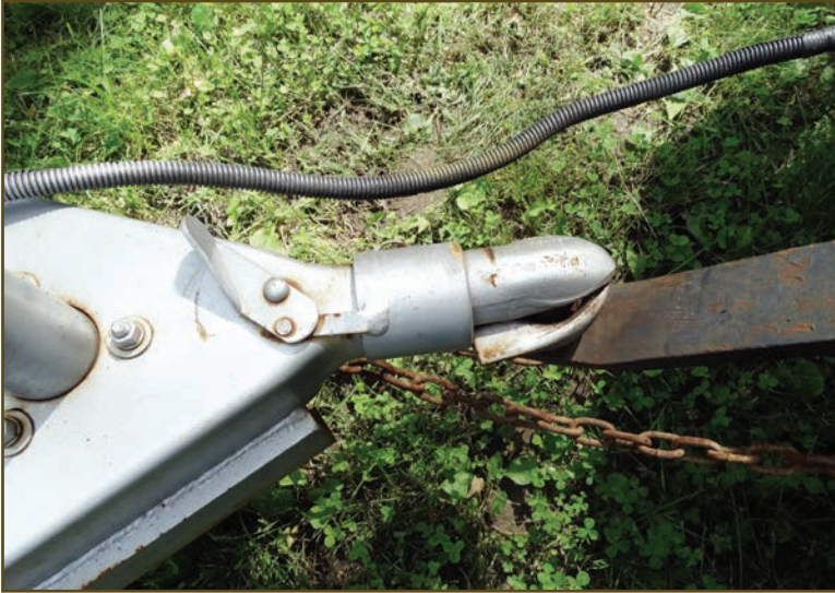
Always check and recheck couplers. You also need a retainer pin or bolt to keep the coupler closed — otherwise, one bump or sudden stop will open the coupler and allow it to come off the ball.
