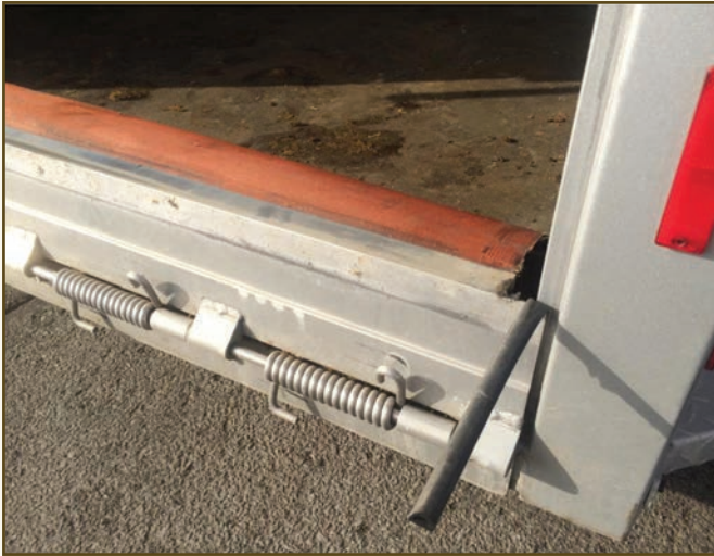
The ramp fell off this trailer, exposing the springs.
