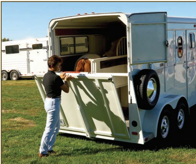
This ramp load trailer with a broken spring assist requires the handler to lift the ramp from the middle. If a horse tries to escape, a person could be crushed underneath the ramp. Make sure ramps are in good working condition to avoid these situations.
