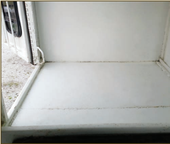
Make sure all parts of the trailer are solid, including this manger. Panicked horses could jump up on the manger, so you want it to be solid enough to withstand the impact of a hoof and the horse's weight.
