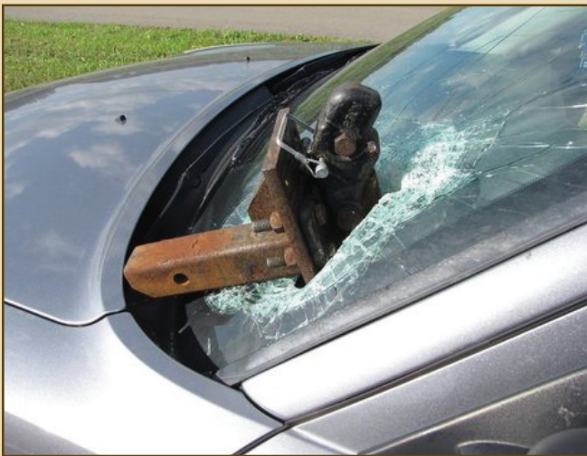
This ball mount disconnected from a receiver and hit the windshield of a car that was following the tow vehicle.
