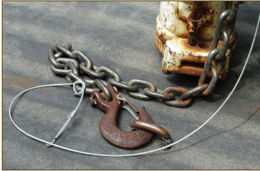
This damaged breakaway brake system cable might snap before it is able to pull out the pin.
