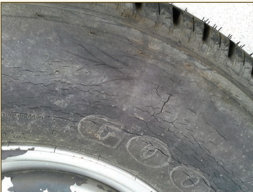
This trailer tire is in poor condition because it is old. Whether the tire has any tread is irrelevant; this tire should not be in service.
