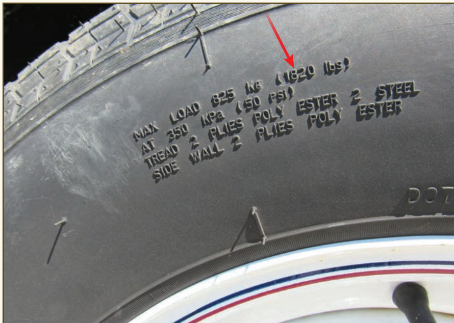
Trailer tires indicate the maximum pressures and weights they are designed to carry. (Top) This tire can carry up to 6,175 pounds when inflated at 110 psi. Note that it can carry less when used in combination with another tire. (Bottom) This tire can carry up to 1,820 pounds when inflated at 50 psi.
