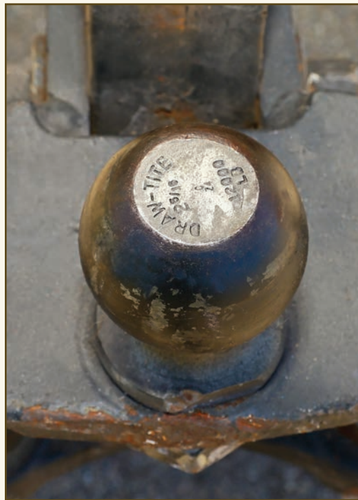
A 12,000-pound, 2 5/16-inch ball on a weight-distributing mount.
