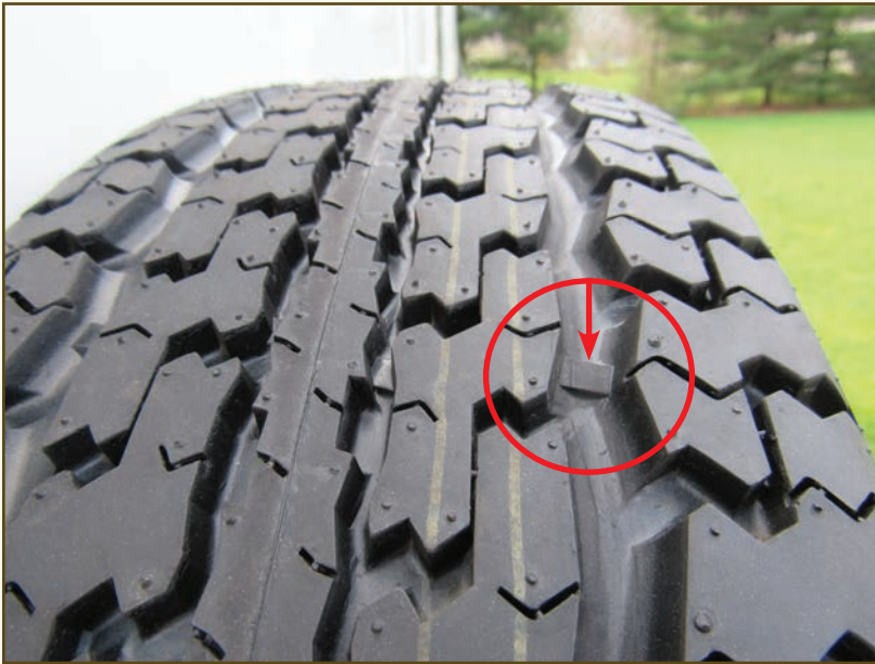
New tires have wear bars. Once the tire has worn to the depth of the bar, it is time to replace the tire.
