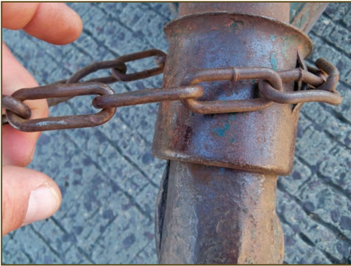
Lawsuits and settlements are often won or lost based on the condition of the equipment. (Left) A chain that is stretched. (Right) A ball that is worn. Driving with badly worn equipment makes it difficult to defend your claim.
