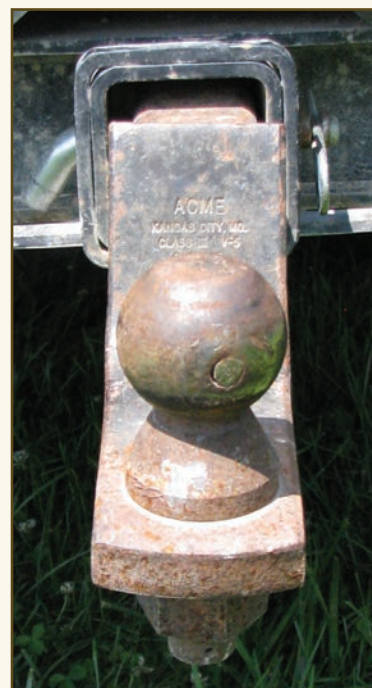
This insert is too small for the receiver and the ball is worn.
