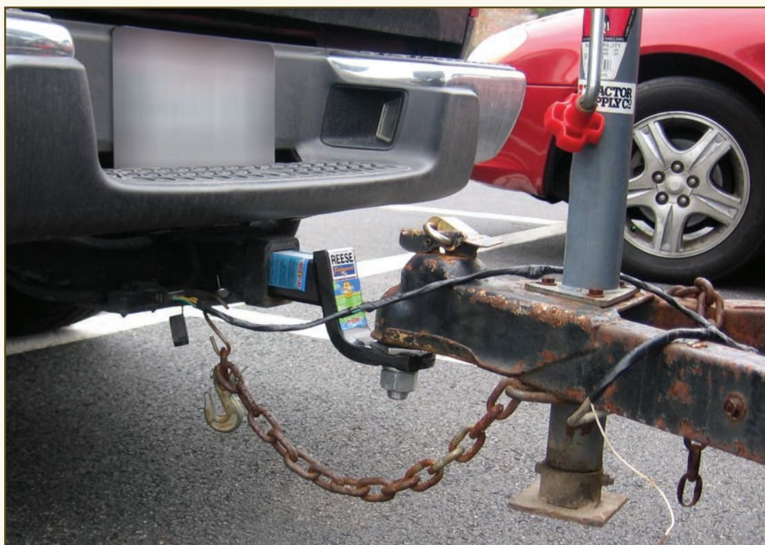
Only one safety chain is connected and it's only connected to a piece of wire, which would never hold the weight of an uncoupled trailer.
