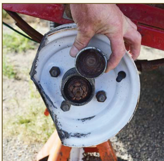
(Right) What's a little dirt (or water, or salt) going to hurt? The dust cap on this axle bearing has fallen off, which means water and dirt can quickly contaminate the bearings and cause it the wheel to fail prematurely. (Left) Pay attention to properly maintaining wheel bearings. Neglecting them can ruin the wheel or lead to real problems on the road.
