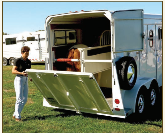
This ramp load trailer with a functional spring allows the handler to easily lift the ramp while remaining at the side well out of the kicking zone. Make sure ramps are in good working condition so you can stay safe.
