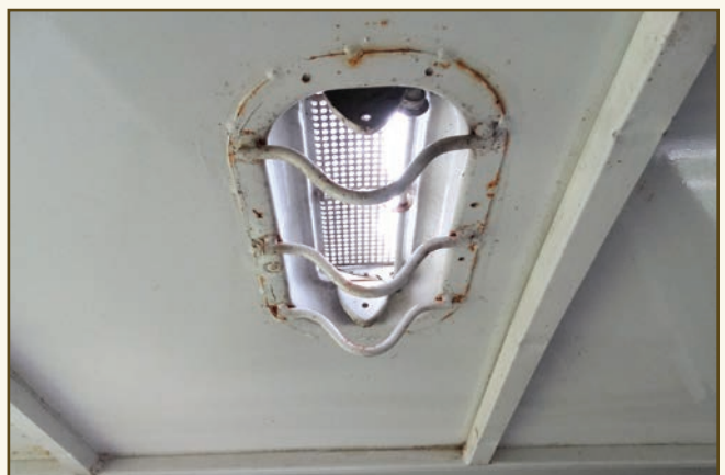
Trailer ventilation is notoriously bad — more vents are always better. Make sure trailer vents and windows operate properly so your horses can get adequate fresh air during transport.
