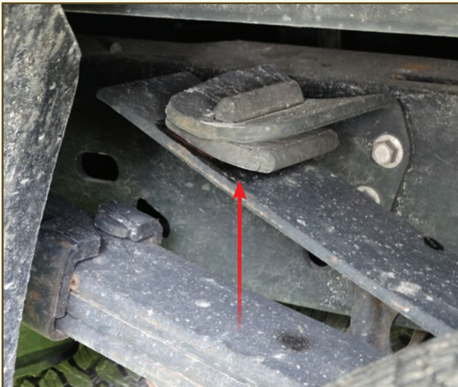
A quick way to determine if you have too much tongue weight on the tow vehicle, is to check on the helper (or overload) springs in the rear suspension of the truck. (Top) When the bumper stops sit off of the helper spring, then the back end of the truck is not overloaded. (Bottom) When the bumper spring is touching the bumper stop, you are approaching the maximum designed load.
