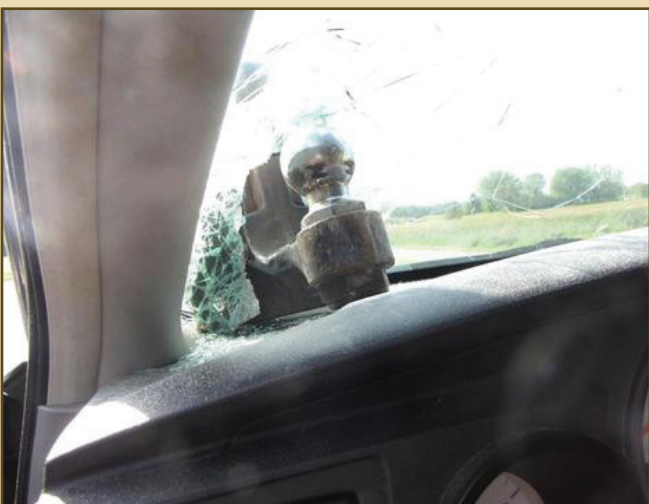
This ball mount disconnected from a receiver and hit the windshield of a car that was following the tow vehicle.
