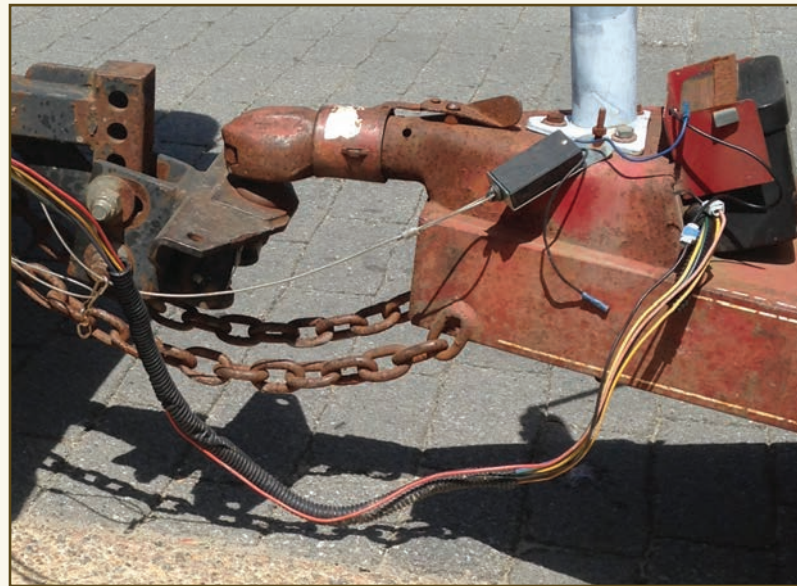
The coupler on the trailer and ball must fit together like a ball and socket. The ball and the coupler shown here are not seated well together — this is a poor connection.
