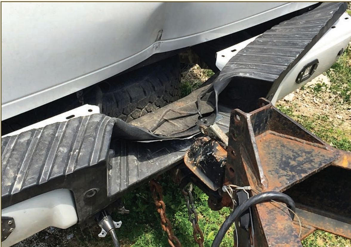
This trailer's coupler came undone, but the safety chains kept the trailer connected. When this happens, the trailer often damages the back of the truck, but that is obviously better than letting the trailer run into nearby vehicles.
