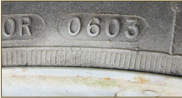
You can tell how old a tire is by looking at the DOT identification on the tire. The first two numbers are the week (1-52) and the last two numbers are the year. (Top) This tire was manufactured in the sixth week of 2003. (Right) This tire was manufactured in the eighth week of 2005.
