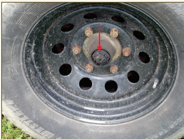
(Right) What's a little dirt (or water, or salt) going to hurt? The dust cap on this axle bearing has fallen off, which means water and dirt can quickly contaminate the bearings and cause it the wheel to fail prematurely. (Left) Pay attention to properly maintaining wheel bearings. Neglecting them can ruin the wheel or lead to real problems on the road.
