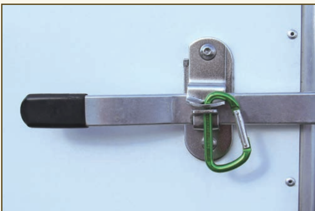
Cheap aluminum carabineers are better than nothing — but that's about all you can say about them.
