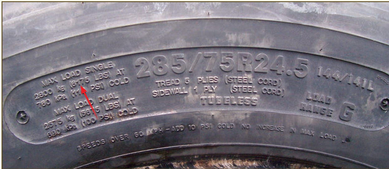
Trailer tires indicate the maximum pressures and weights they are designed to carry. (Top) This tire can carry up to 6,175 pounds when inflated at 110 psi. Note that it can carry less when used in combination with another tire. (Bottom) This tire can carry up to 1,820 pounds when inflated at 50 psi.
