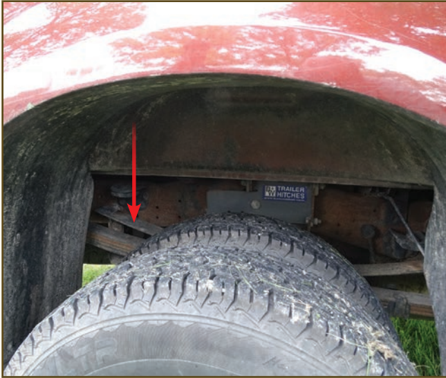
A quick way to determine if you have too much tongue weight on the tow vehicle, is to check on the helper (or overload) springs in the rear suspension of the truck. (Top) When the bumper stops sit off of the helper spring, then the back end of the truck is not overloaded. (Bottom) When the bumper spring is touching the bumper stop, you are approaching the maximum designed load.
