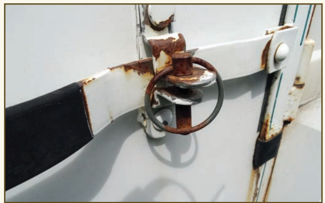
Properly maintain all latches on your trailer. You should add additional locking pins to ensure latches do not come free during transport.
