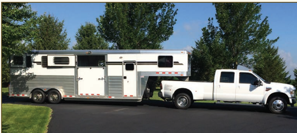
A horse trailer with a gooseneck rig couples to a ball above the rear axle of the truck (inside the truck bed). Note that a gooseneck rig is different than a fifth wheel. A gooseneck uses a ball, a fifth wheel uses a flat "kingpin" receiver similar to a semi.
