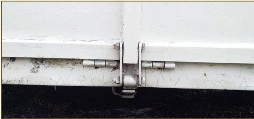
This ramp has a spring assist as a separate leaf spring attachment. Such designs are often found on older trailers.
