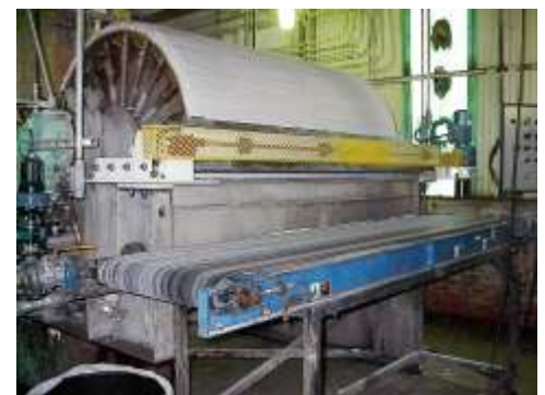
EDG-trac™ Knife Advance retrofitted to Eimco rotary vacuum drum filter
