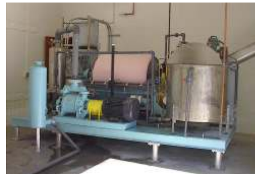
Complete skid-mounted 3'x4' Pre-Coat RVDF system with vacuum system, pre-coat system, and full automation
