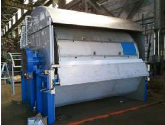
Remanufactured rotary vacuum drum filter by TriStar LTD. One of a pair of completely rebuilt filters including new drives, new hood, and wash system.
