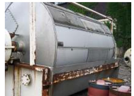
Rotary vacuum drum filter before rebuilding
