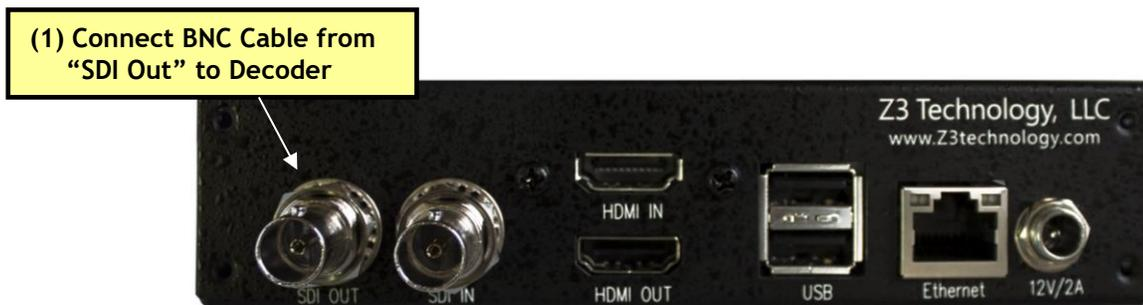
**Figure 20 DME-05 Rear Panel ASI Output Connection**
