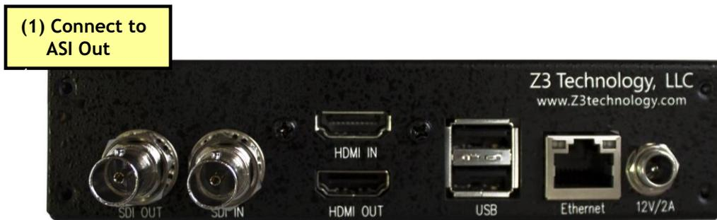
**Figure 34 Z3-MVE-250 Rear Panel Example Encode Connections**
