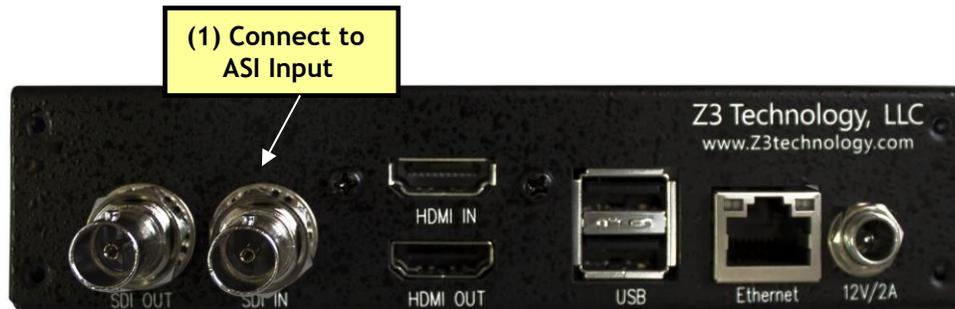
**Figure 42 DME-05 Panel ASI Decode Connection**
