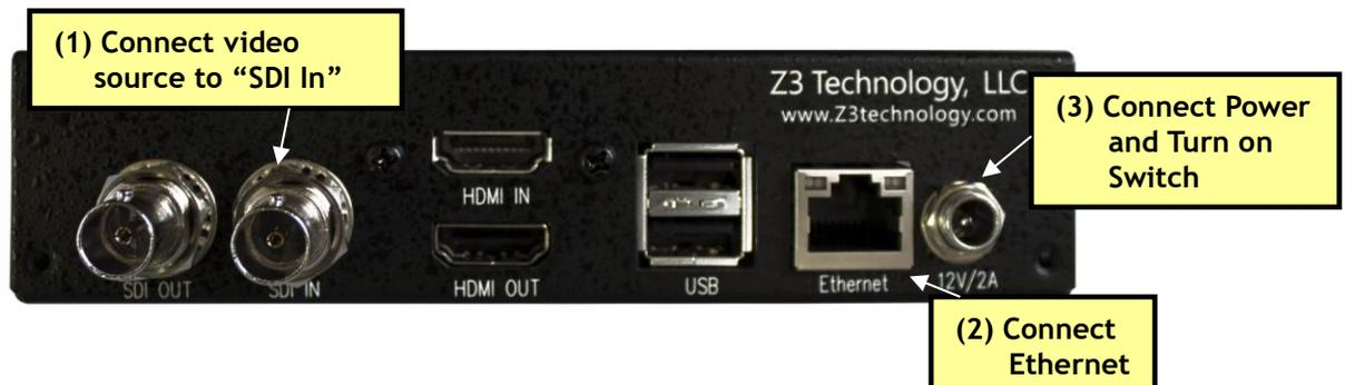
**Figure 3 DME-05 Rear Panel SDI Encode Connections**
