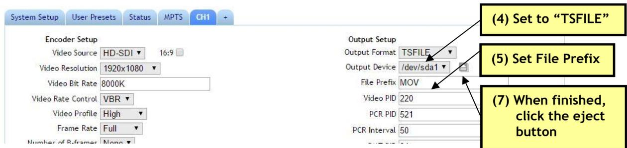
**Figure 32 CH1 Tab Configuration - TSFILE**
