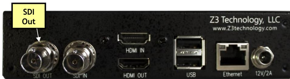
**Figure 50 DME-05 SDI Output Connection for Decode**
