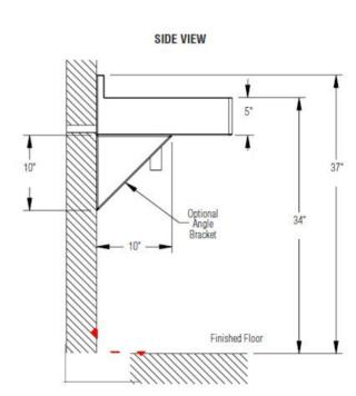
Engineering Specification: 16 gauge, type 304 stainless steel single wash sink. Exposed surfaces polished to a satin finish. Supported on (2) wall brackets and clips.1-1/2 Welded drain
