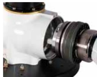
**Easy Installation** and maintenance due to removable blade cartridge.
