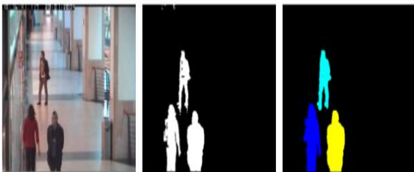
Figure.2: From the left to the right: original image, result obtained after background subtraction and finally after connected components gathering.
