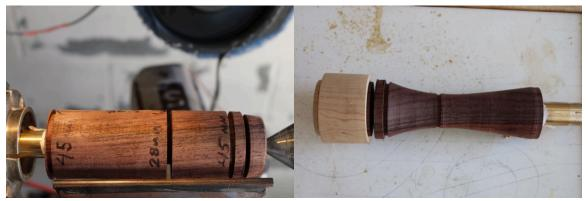
I have made a drilling jig that requires that I turn a taper on the waste area above
