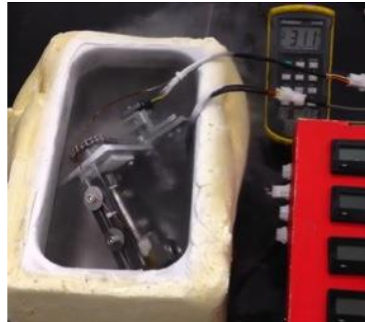
Stepper Motor Controlled Valve Testing in LN2
