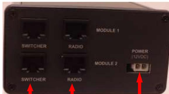
Connect cable supplied with C412 to RAD port on C250/C251 or C150 here. (2 plcs)
