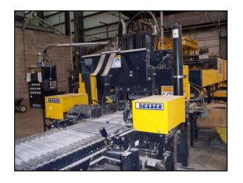
Cured block is processed through the block splitter. Block is inspected for specification conformity prior to being palletized and transferred the inventory storage area.
