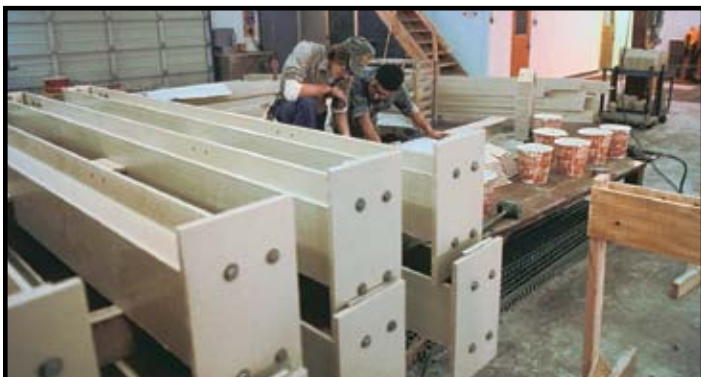
Fabricated Dynaform columns ready for shipment.
