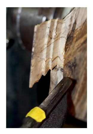
HINT: When cutting wing to final thickness it is better to go a little too thick than too thin, it's hard to recover from too thin. You can always sand down the thick areas.
