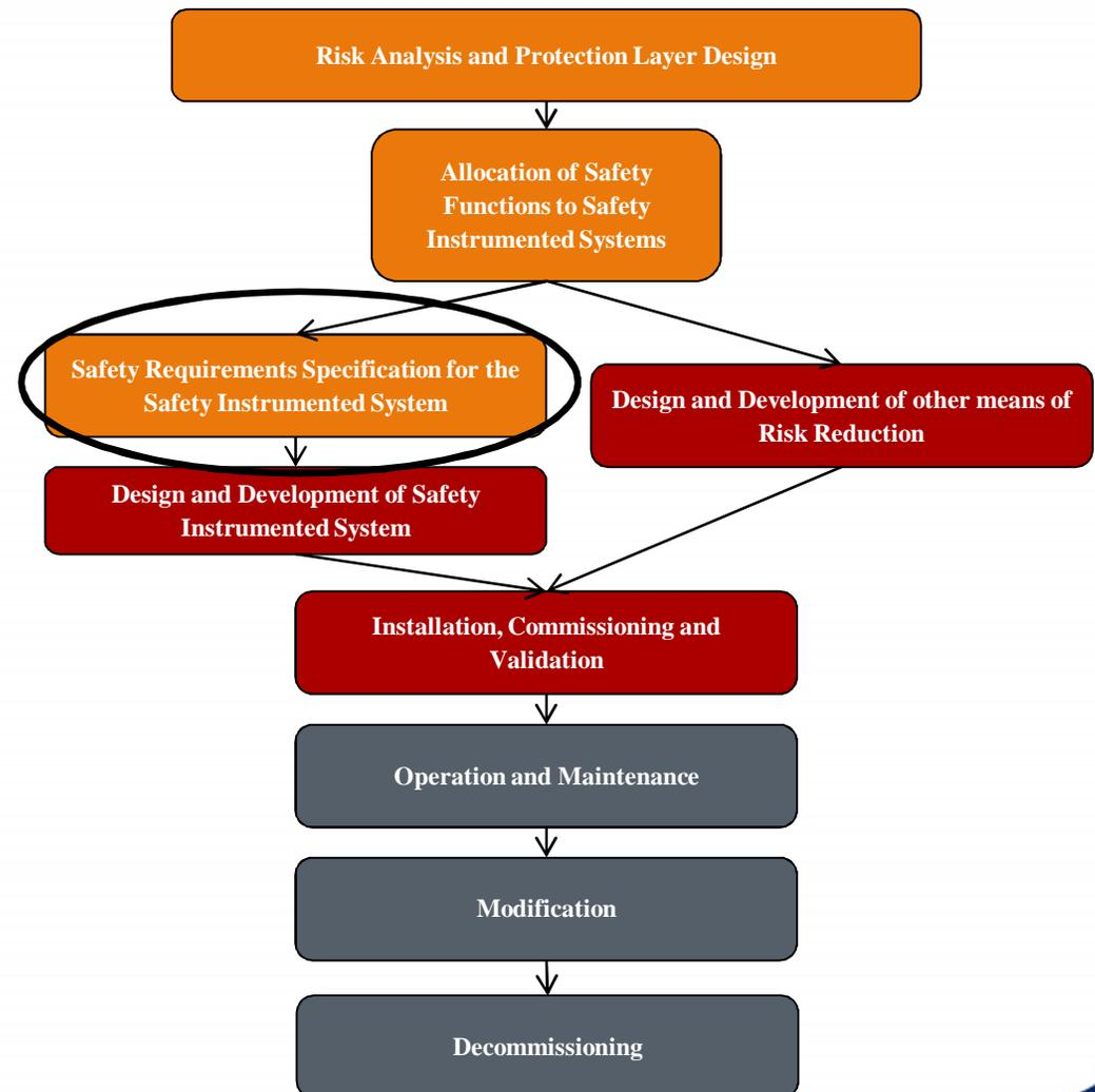
The SRS is the “Interface“ of the process environment in the world of automation
