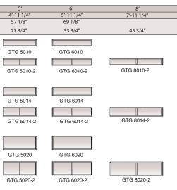
1. Rough Opening Width=Unit Dim. Width + 3/4" 2. Rough Opening Height = Unit Dim. Height + 1/2" 3. Glass Option: Clear / Inner Grille / Art Glass
