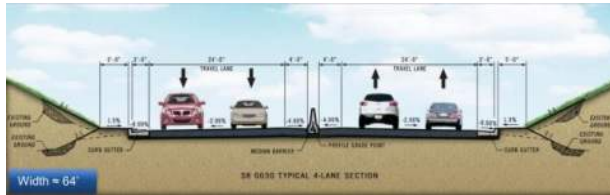
Figure 6: Typical 4-Lane Section (Alternative 1)
