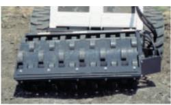
Drum oscillation keeps the roller in contact with the surface on uneven terrain.
