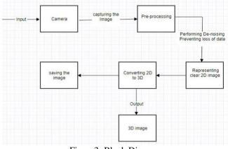
Figure3: Block Diagram
