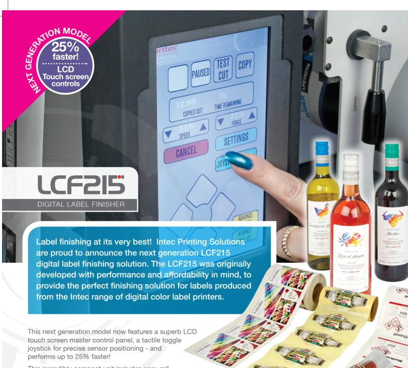
This incredibly compact unit includes easy roll loading for lamination, contour cutting, matrix removal and slitting. Combining robust engineering with precision registration, with the ability to select from one to three registration points, it ensures complete cutting accuracy and finishing performance.
