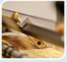
Slitting blades allow for roll slitting, at any width, with up to 5 blades. (3 blades supplied as standard with machine).
