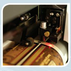
Optical sensors read up to 3 registration marks which ensure the best accuracy in the industry.
