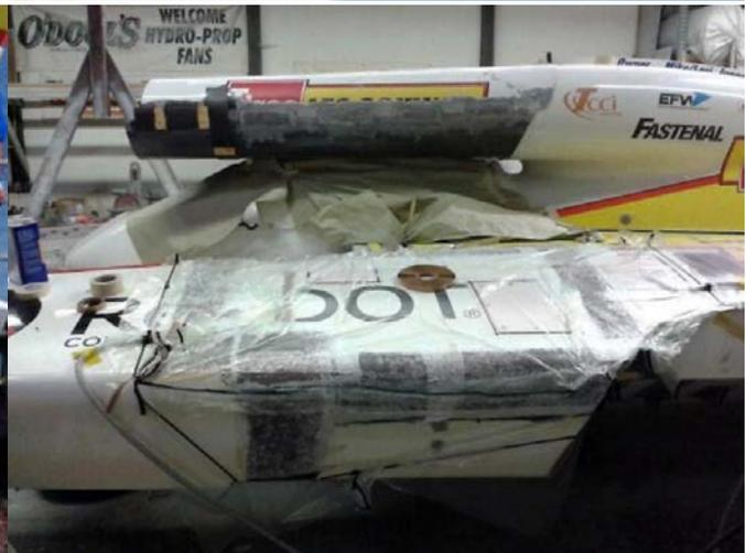
**#9 Les Schwab-RedDot** - The Jones crew is once again busy with repairs to the race boat after a steering failure in San Diego contributed to a spinout causing damage to the several areas of the boat. The saltwater scoop was tore off, the rudder bracket failed, and left sponson/skidfin area suffered damage. Above, shots of the #9 damage at San Diego. ~ Mike Parker photo
