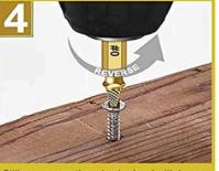
Still reverse use the extractor head with lower speed and take out the brocken bit
