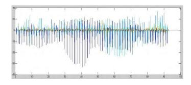
Figure 10. MFCC plot for the speech waveform input after pre processing
