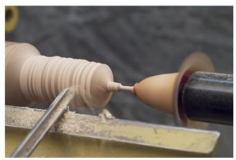
I continue with the same technique as before to remove wood and begin to thin the stem. Cutting downhill from left to right with bevel suported cuts (above and right)
