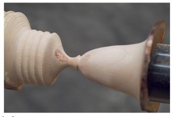
14 The soft pith area is visible in the waste wood portion and also in the bottom of the goblet. This will be turned away as we turn the stem but the area in the goblet will need to be delt with.
