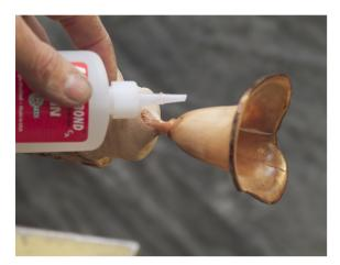
In this photo you can also see the cracks in the side of the goblet, I have chosen to reinforce the goblet with CA glue. With the lathe turning at a very slow speed I allowed the glue to coat the entire goblet both inside and out. Leaving the lathe running I went to lunch to give the glue plenty of time to dry.
