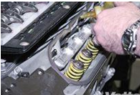
Engine Build - installing springs. Photo courtesy of Super Chevy online magazine.
