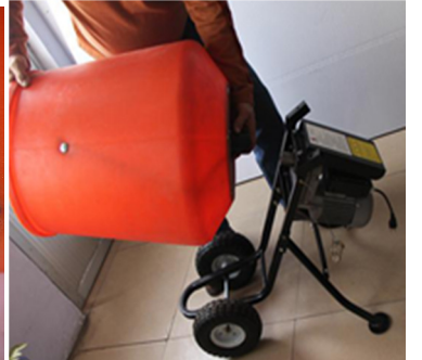
8. Slide on drum. Line up 1/2" hole.
