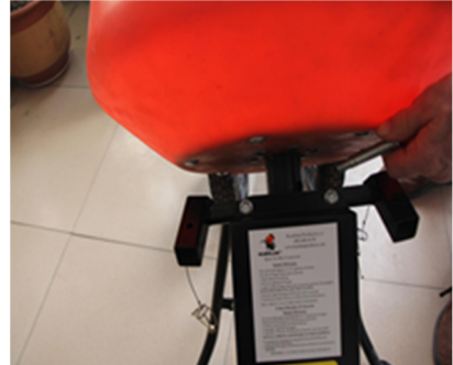
9. Install 5/16" bolts and lock nut
