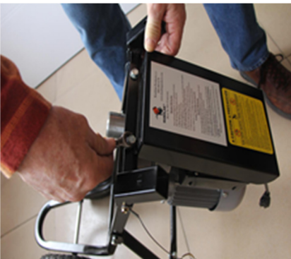
6. Install metal cover on gear motor with 5/16x3/4 bolts.
