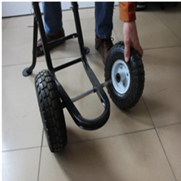
4. Install wheels and axle. Put on washer and cotter pin.
