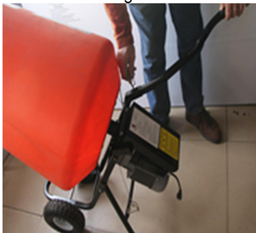
10. Install handles and clevis pin with lanyard.
