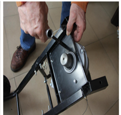
5. Install gear motor with flat washer, spring washer and nuts Tighten with 10 MM wrench..
