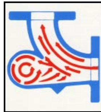
Figure 1: A cross section of the new type of elbow in use at Chromalloy. Suspended material coming from the right forms the slowly revolving soft mass of product suspended in air. The soft ball revolves slowly, and is self-renewing as some new product is added at the top and particles leaving the bottom deflect and join the main product stream
