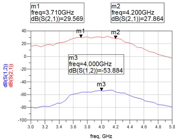
Figure 5: The  $S_{21}$  and  $S_{12}$  of the LNA.
