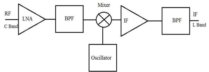
Figure 1: Low noise block downconverter diagram
