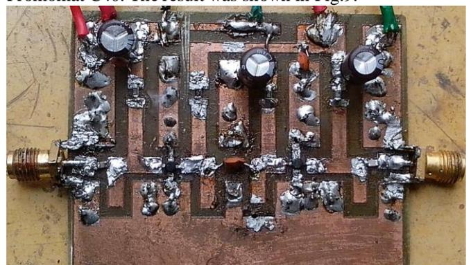
Figure 9: The fabricated LNA
