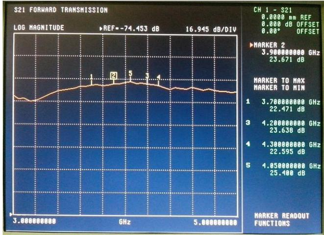
Figure 10: The gain of the LNA
