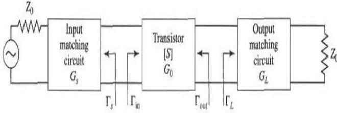
Figure 3: The diagram of a single stage amplifier stage.
