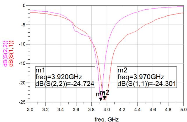
Figure 6: The  $S_{11}$  and  $S_{22}$  of the LNA
