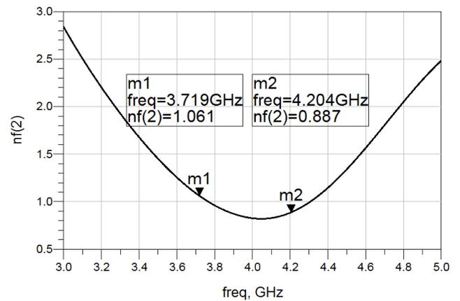
Figure 7: The noise figure of the amplifier
