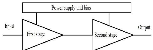
Figure 2: Diagram of two-stages cascade LNA
