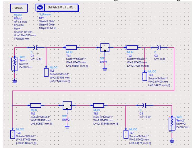
Figure 4: Schematic of the two-stages cascade LNA
