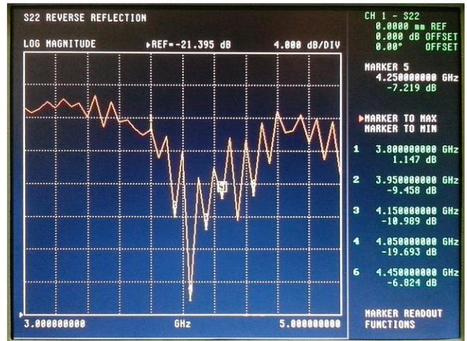
Figure 12: The output reflection coefficient
