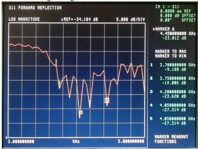
Figure 11: The input reflection coefficient  $S_{11}$
