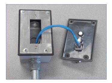
2. Route the Ethernet cable through one of the outlets and into the back of the keyport.
