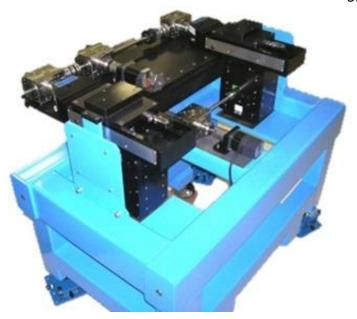
This custom BNL two degrees of freedom High Precision Motorized Optical Table was designed to hold a scientific instrument. The system base was made of a welded steel frame with a powder coated finish. Frames were filled with sand to reduce the table natural frequency and provide passive damping. When in use, the table rests on four machinery feet. When in transport, the feet are retracted and casters allow for easy handling. To learn more about BNL please go to: http://www.bnl.gov/ps/
