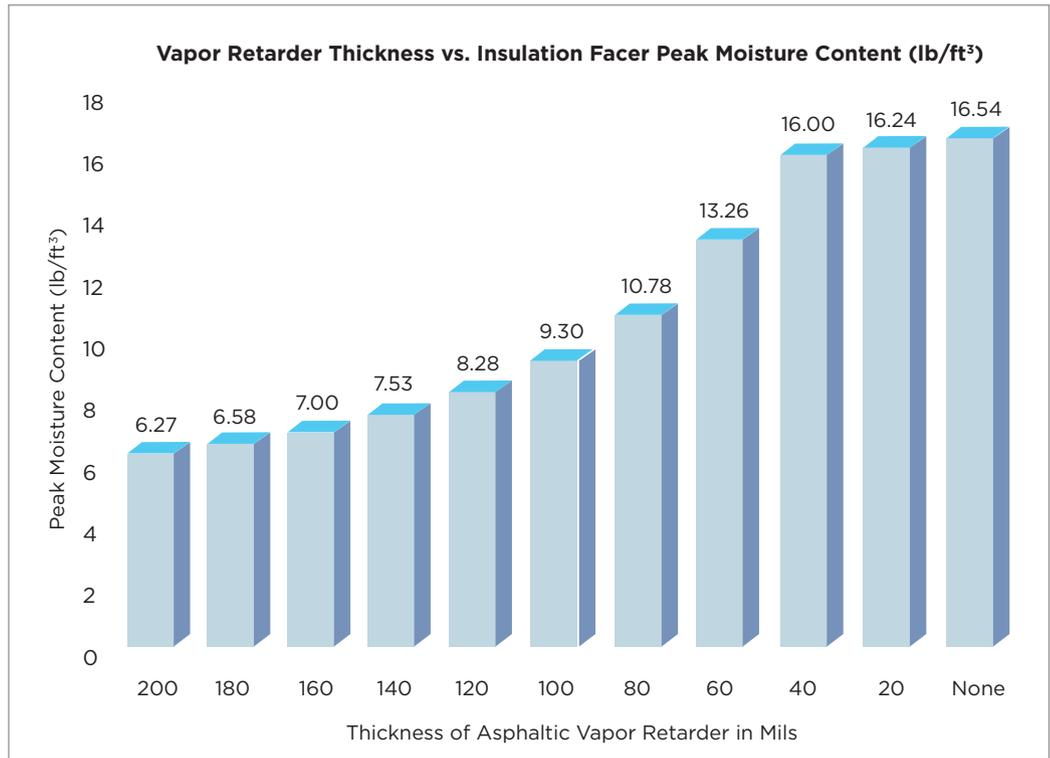
Figure 3: This graph shows simulation results for a roof modeled in Chicago. The results show the peak moisture content over time in a facer in the insulation system. Typically in northern climates, this will be the topmost facer under the roof membrane during the end of the winter season.
