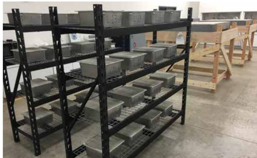
Photo 2: Concrete slabs and pan specimens, both regular weight and lightweight structural concrete, in SRI Consultants’ laboratory in 2016
