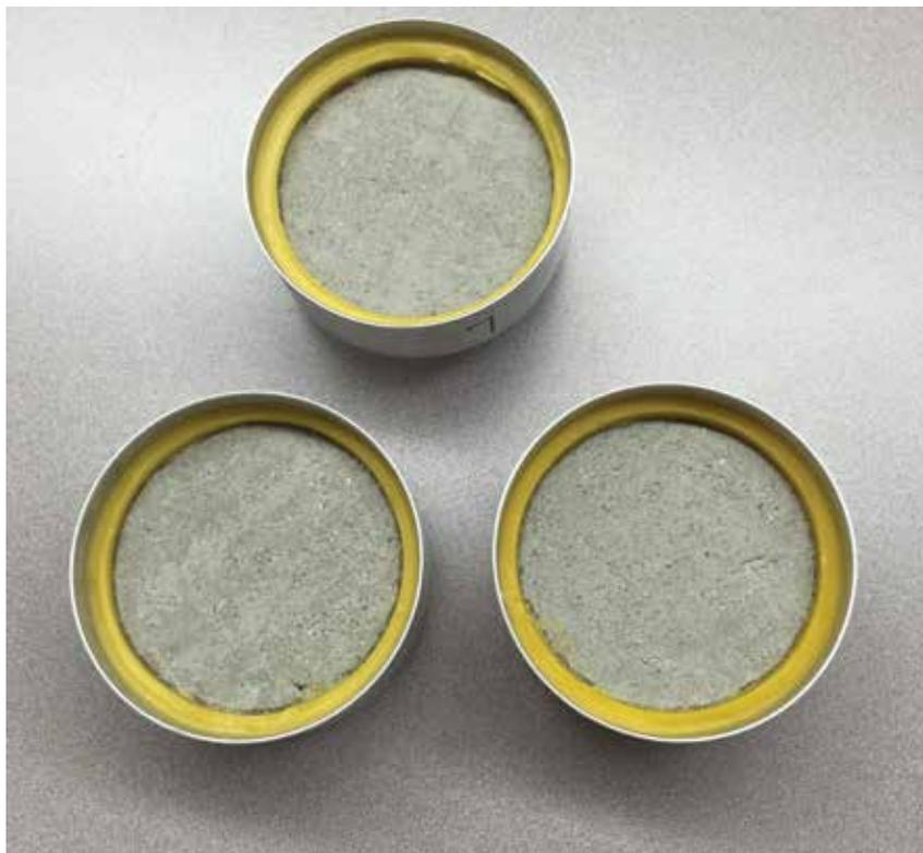
Photo 5: Concrete specimens prepared for ASTM E96 water vapor transmission testing
