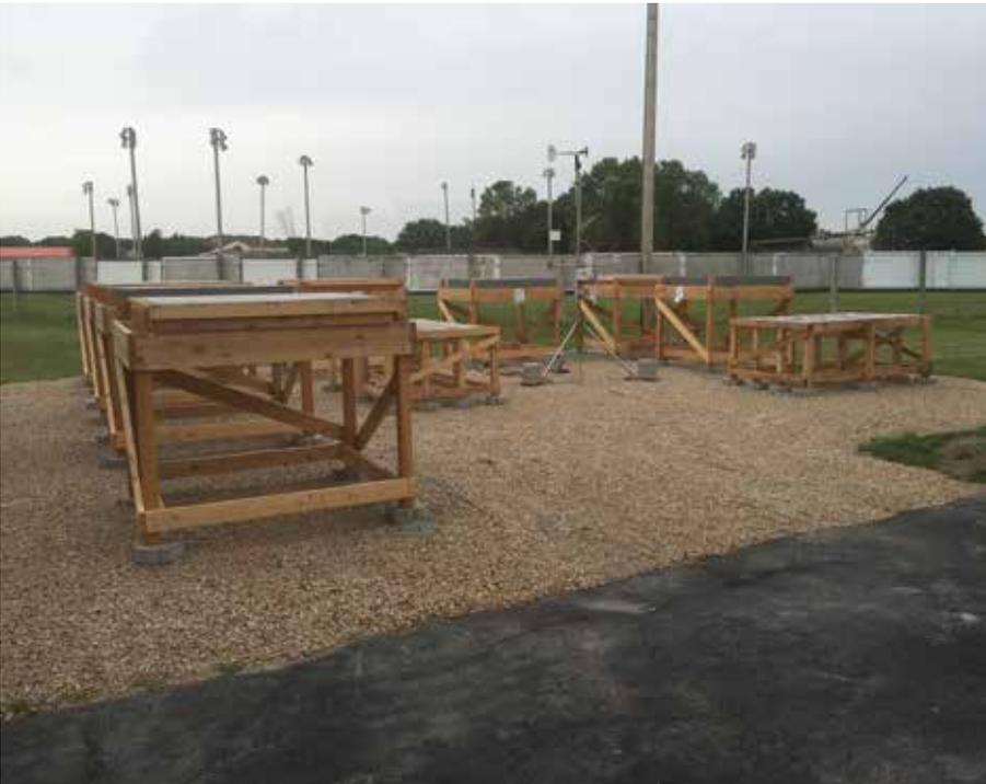
Photo 4: The poured concrete slabs and pan specimens, both regular weight and lightweight structural concrete, during outdoor weathering
