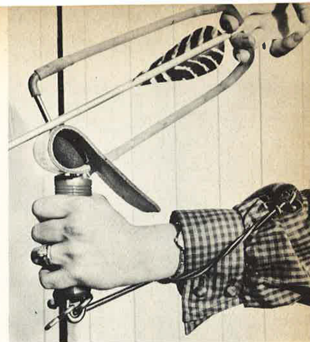
Arrow is nocked on straight steel rod inserted between protective bits of rubber. Note padded wrist brace.
