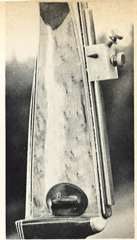
The sight which Tone used to win the Canadian title is easily adjustable for windage, elevation, uses a pin.
