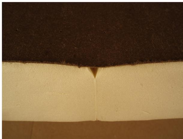
Knit line and V-groove close-up (after conditioning)
