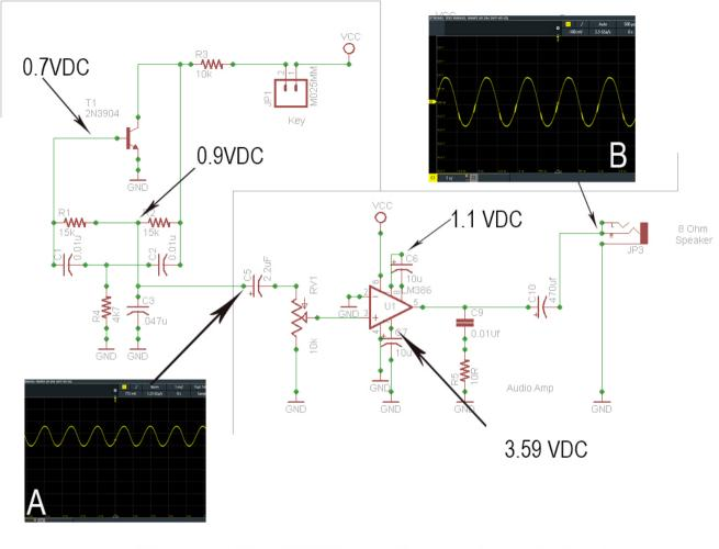
Voltages are typical for an 8 VDC VCC, test conditions are, key down, speaker attached, Volume at mid point. Waveform 'A' is for the Twin T output, while 'B' is after amplification.
