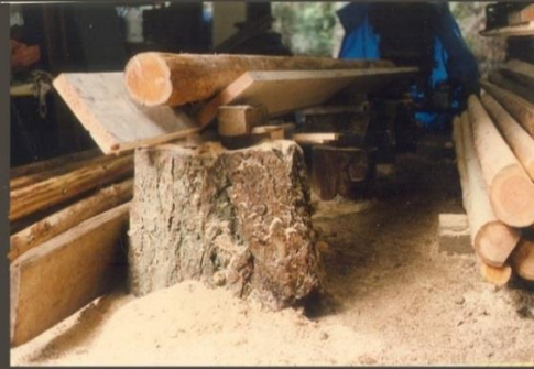
Blocked up rafter ready for milling
