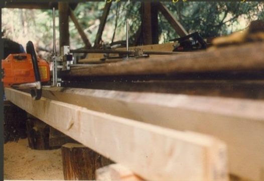
The rafter was cradled in the V. The plank was made flat. The plank was held fast to the rafter with short nails that would clear the cutting teeth of the saw.
