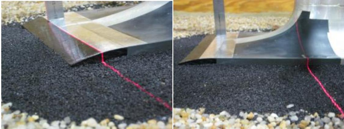
Figure 7. Gravel level after flume test for 12.7mm high elevation with a 12.7mm high straight-sided curved leading edge ramp. No scour is observed (8).
