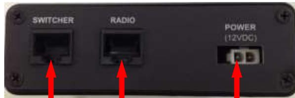
Connect cable supplied with C411 to RAD port on C250/C251, C150 or C151 here.
