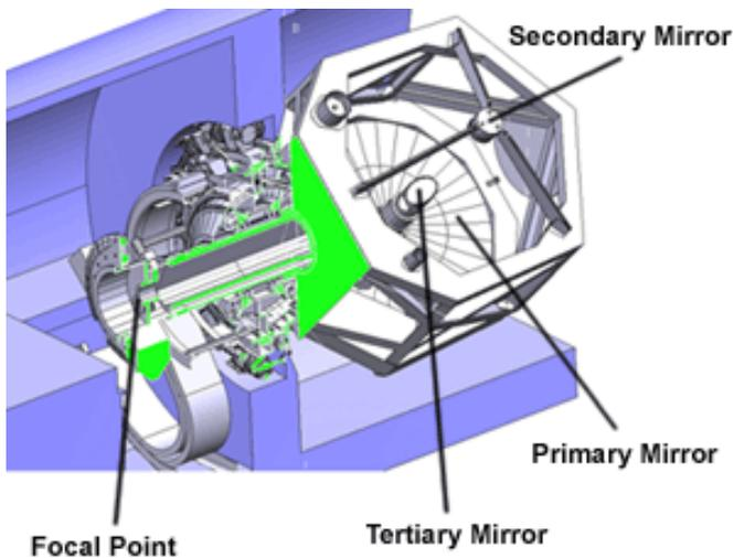
Figure 2 – The SOFIA 2.7-meter IR telescope in its mounting. (NASA)
