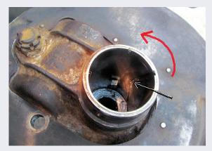
To remove the sleeve, engage the puller button in the sleeve grease hole, then twist the sleeve completely in the correct direction to allow the sleeve's raised dimple to release from its retaining hole at the outer axle housing end. Continue to twist and pull, or tap firmly with a mallet, on the puller bar as the sleeve twists free of the axle housing.
