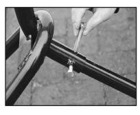
Step 5 Put in Bolt to Hold Main Frame to Draw
