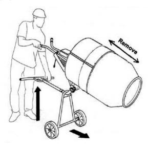
When tilting the drum to pour material, do so in a very smooth manner. This keeps the mixer balanced and upright.
