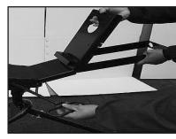
**Step 8**Connect Gear Motor Mounting Base to Swivel Bracket Using the Pivot Pin.
