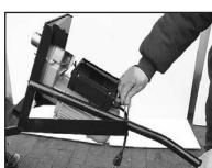
**Step 11**Install the Back Dump Handles if Desire For Your Operation.
