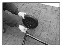
**Step 1**Install Wheels on Lower Frame Unit
