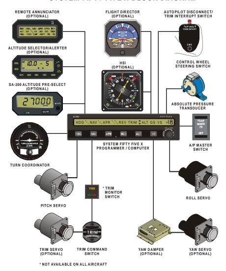
Fig. 2-1. System Fifty Five X Block Diagram
