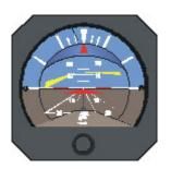
For proper flight technique, the system presentation requires the pilot to roll and pitch the aircraft toward the steering command bars until the delta-shaped reference is tucked into the steering command bars, indicating that commands have been satisfied. For example, if the display is up and left, the pilot would be required to establish a left turn, pitch-up attitude.
