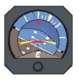
As bank angle and vertical speed approach the required amounts, bank angle and pitch-up attitude are shallowed. When the delta reference and the steering bars are matched the commands have been met. Thereafter, it is necessary to maneuver the aircraft to keep the display elements matched in order to accurately fly the programmed modes.
