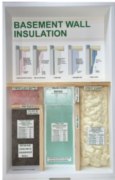
BASEMENT WALL INSULATION
