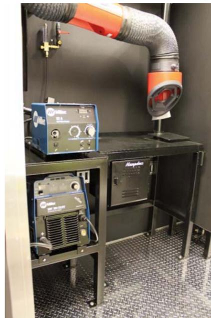
Ventilation Exhaust and Bench Setup
