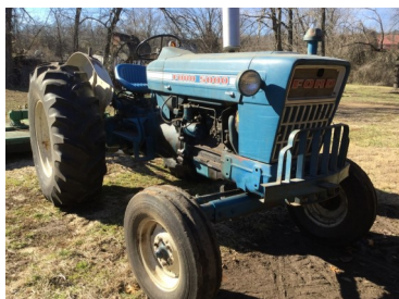
Ford 5000 diesel tractor, 52 hp, 4-way hydraulics, tach shows 5725 hrs
