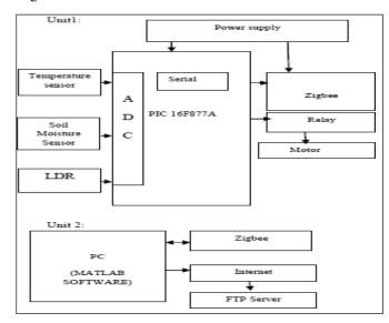
Fig.1: Wireless sensor unit and Information unit
