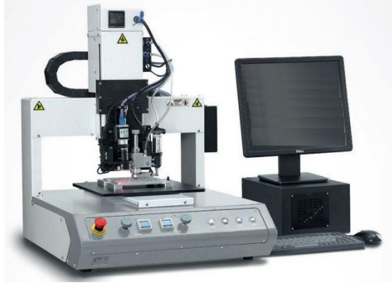
Non-contact NanoLiter volume Live Cell Dispensing Robot Optional Temperature and Humidity enclosure not shown
