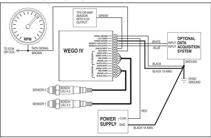
Figure 3 – Typical Dyno Hookup for WEGO IV Dual Channel
