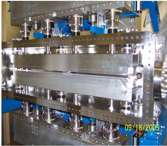
Figure 7. The fully opened jaw (19 mm) at chamber can ease the magnet for measurement and shimming
