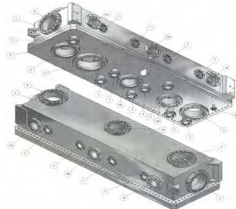
Figure 6. Chamber drawing shows a full-size removable front panel and multi build-in ports
