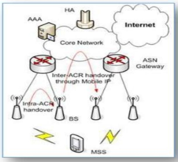
**Figure 1: Network Architecture of Mobile WiMAX [4] [6]**
