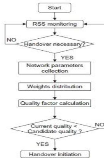
Figure 3: Hasswa et al. VHD heuristic algorithm [18]
