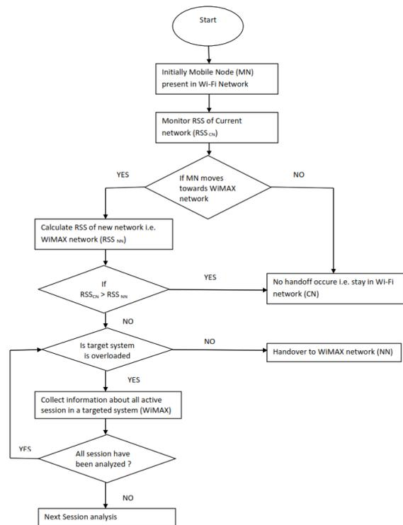
Figure 4: Proposed algorithm flow chart for VHD
