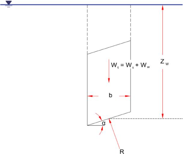
**Figure 1 – Hydrostatic condition**
