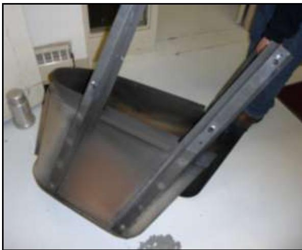
Fig. 17. HIRSS Extender from UH-60 before blasting with Type VIII PMB (inside) Fig. 18. HIRSS Extender from UH-60 after blasting with Type VIII PMB (inside)
