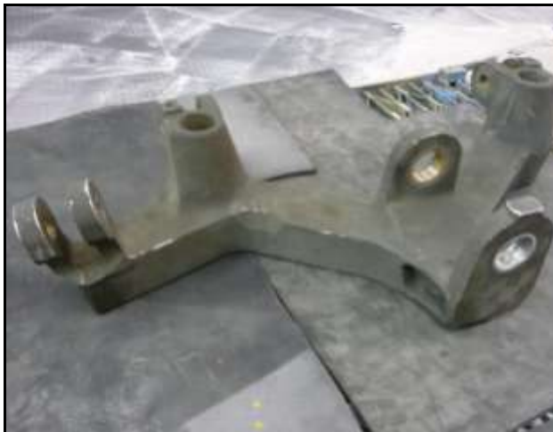
Fig. 21. AH-64 bell crank before blasting with the Type VIII PMB
