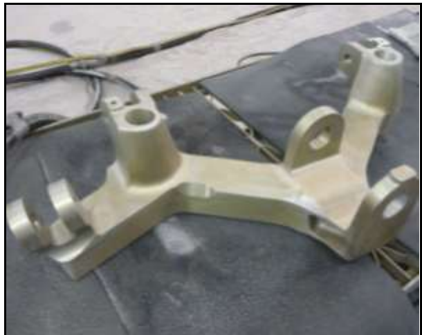
Fig. 22. AH-64 bell crank after blasting with the Type VIII PMB
