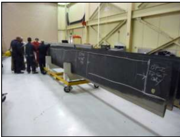
Fig. 6. Note chalk marked areas for blasting
