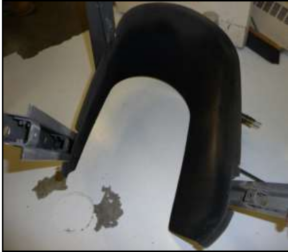
Fig. 19. HIRSS Extender from UH-60 before blasting with Type VIII PMB (inside)
