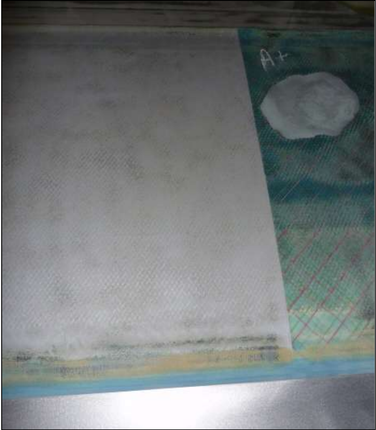
Fig. 13. Here is an excellent example of how good the Type VIII PMB removes coatings from composite substrates on the CH-47 rotor blades. The white square section to the left is one of the lightning strike panels. It is a very delicate area on the blade to remove coating from without damaging it. When using the Type VIII PMB, the topcoat only is first removed on the lightning strike panel at a setting of 15 psi. After the topcoat has been completely removed, the pressure is then turned down to 10 psi and blasting continues down to the white lightning strike substrate seen here. The circle to the right of the lightning strike panel is another example of repair work.
