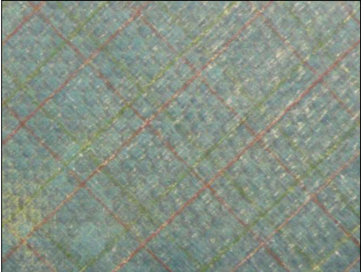
Fig. 5. Another close-up of the CH-47 composite material after stripping with Type VIII PMB
