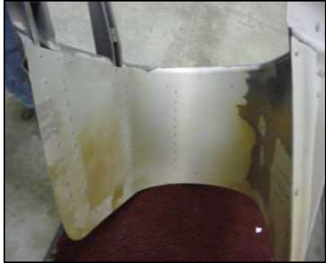
Fig. 20. HIRSS Extender from UH-60 after blasting with Type VIII PMB (inside)
