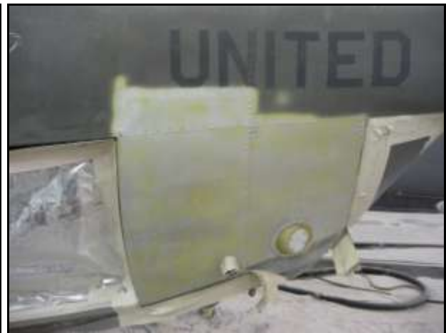
Fig. 32. 0.016" aluminum section after stripping
