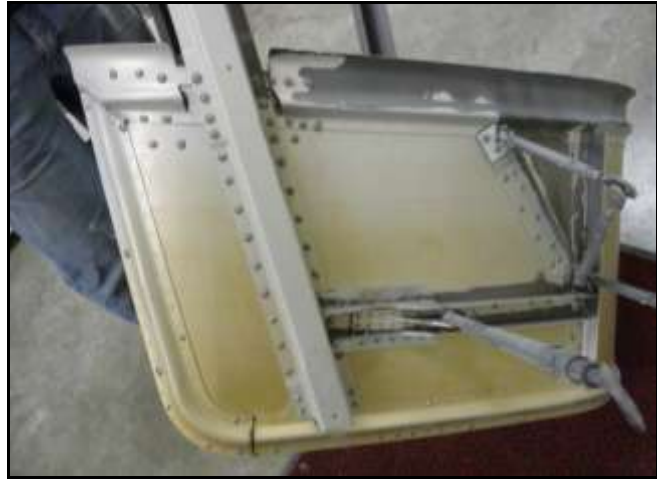
Fig. 15. HIRSS Extender from UH-60 before blasting with Type VIII PMB (outside) Fig. 16. HIRSS Extender from UH-60 after blasting with Type VIII PMB (outside)
