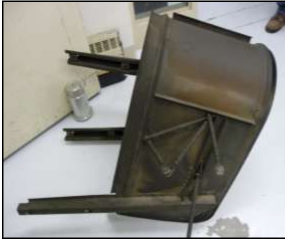
Fig. 15. HIRSS Extender from UH-60 before blasting with Type VIII PMB (outside) Fig. 16. HIRSS Extender from UH-60 after blasting with Type VIII PMB (outside)
