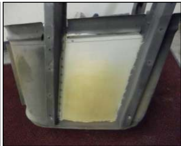
Fig. 17. HIRSS Extender from UH-60 before blasting with Type VIII PMB (inside) Fig. 18. HIRSS Extender from UH-60 after blasting with Type VIII PMB (inside)
