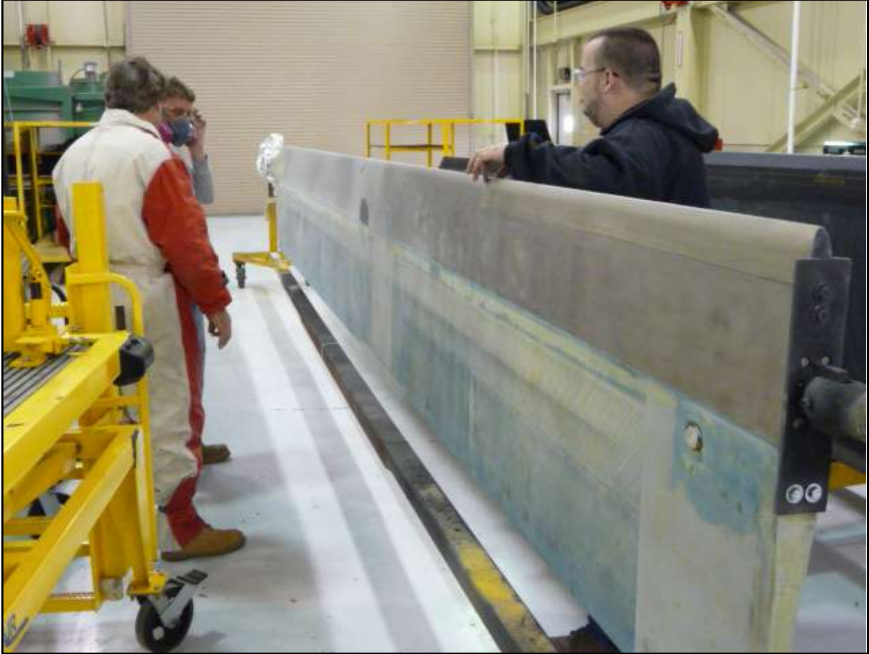
Fig. 10. Vinny, Terry Zurn (Technical Inspector), & Thomas Newman admiring the results of the CH-47 main rotor blade stripped with the Type VIII PMB
